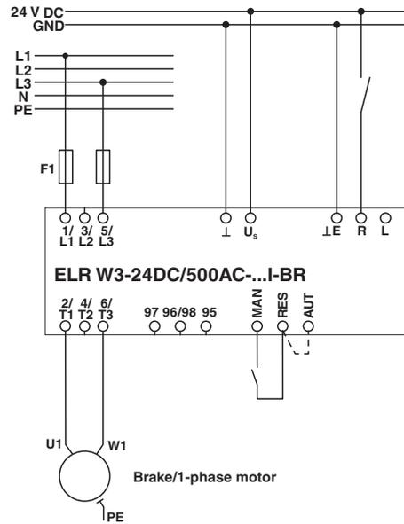
Example circuit for the connection of a brake or a 1-phase motor (L1 + N) Example circuit for the connection of a brake or a 1-phase motor (L1 + L3)
