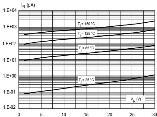
Figure 6. Relative variation of reverse leakage current versus junction temperature (typical values)
