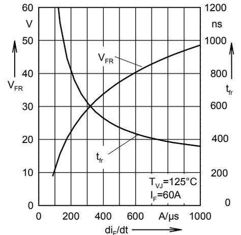
Fig. 6 Peak forward voltage versus  $di_F/dt$ .
