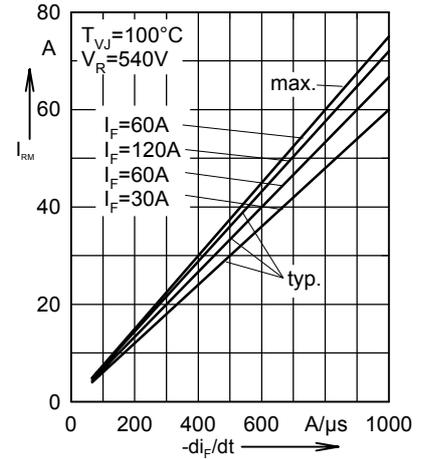
Fig. 3 Peak reverse current versus  $-di_F/dt$ .
