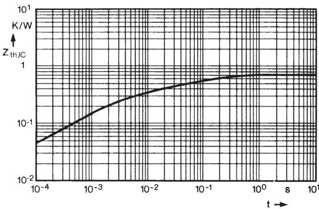
Fig. 7 Transient thermal impedance junction to case.
