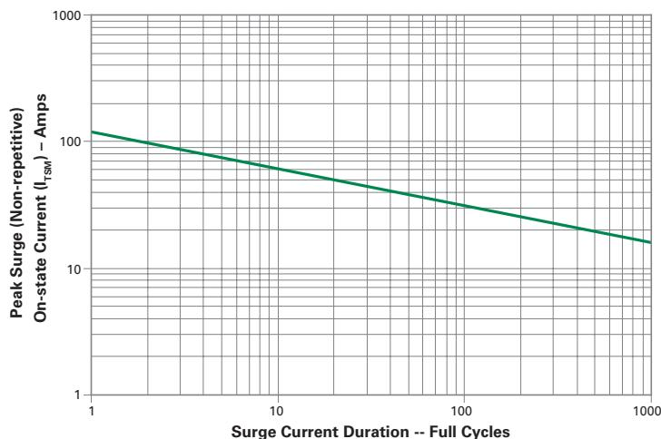
Supply Frequency: 60Hz Sinusoidal
