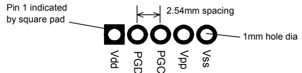
Figure 13. Recommended plate-through connector design
