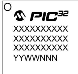
64-Lead QFN (9x9x0.9 mm)
