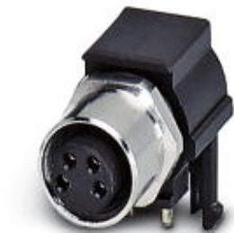
Sensor/actuator flush-type socket, 4-pos., M8, rear/screw mounting with M8 thread, with polarity protection and angled solder connection
