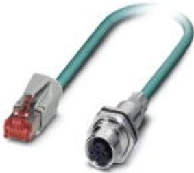
Assembled Ethernet cable, CAT5e, shielded, 2-pair, 26 AWG stranded (7-wire), RAL 5021 (water blue), M12 flush-type socket, rear/screw mounting with M16 thread to RJ45 male connector/IP20, line, length: 0.25 m
