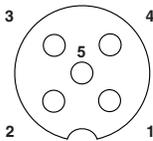
Pin assignment M12, PIN 1: AS-i +, PIN 3: AS-i -,
