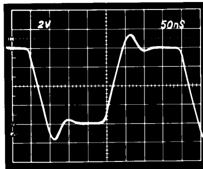
Figure 21b. Inverter Cap Load Large Signal Pulse Response. C_f = 15 pF, C_L = 410 pF
