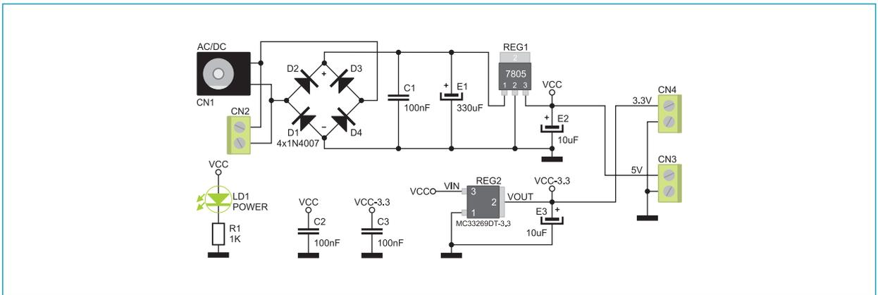
Figure 2: 5V-3.3V REG additional board connection schematic
