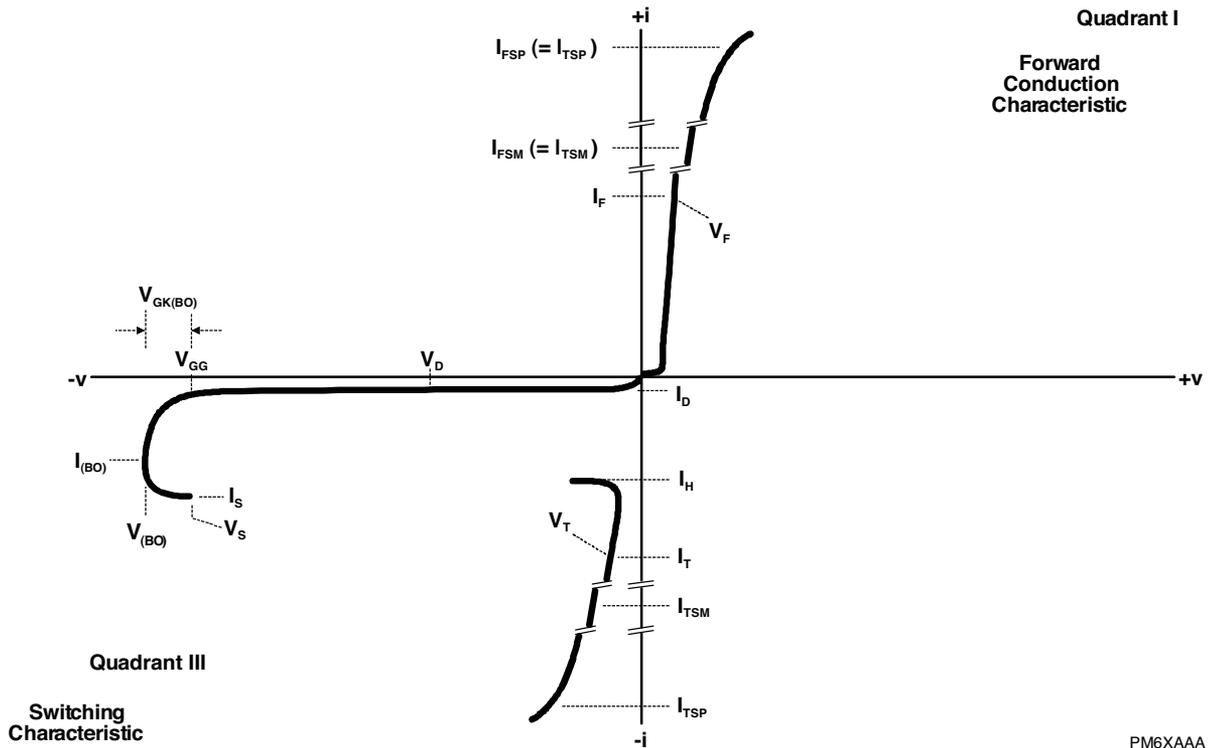
Figure 1. Voltage-Current Characteristic
