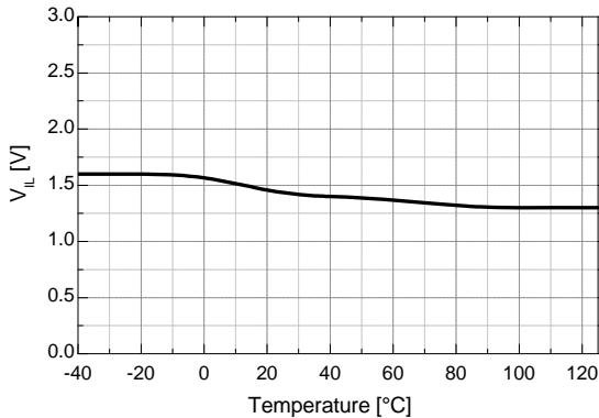
Figure 23. Logic Low Input Voltage vs. Temp.
