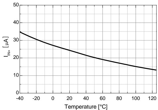
Figure 24. Logic Input High Bias Current vs. Temp.
