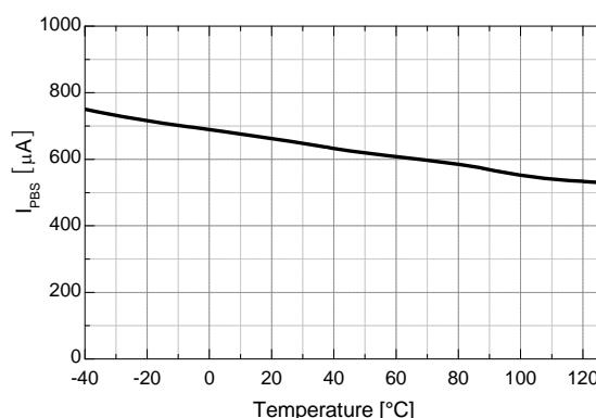
Figure 15. Operating  $V_{BS}$  Supply Current vs. Temp.
