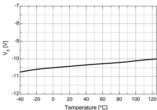
Figure 25. Allowable Negative  $V_S$  Voltage vs. Temp.
