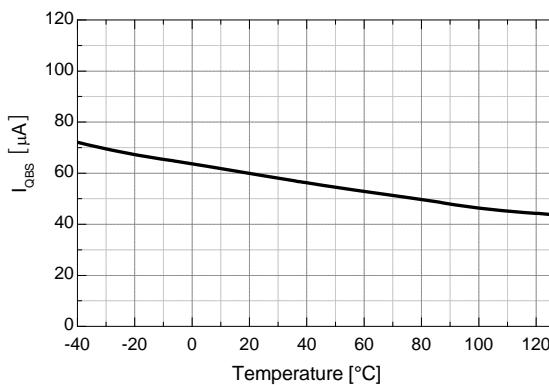
Figure 13. Quiescent  $V_{BS}$  Supply Current vs. Temp.
