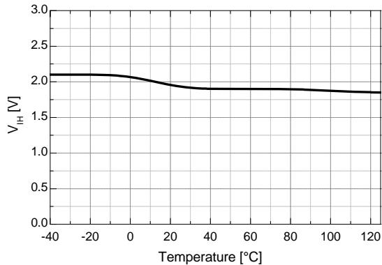
Figure 22. Logic High Input Voltage vs. Temp.
