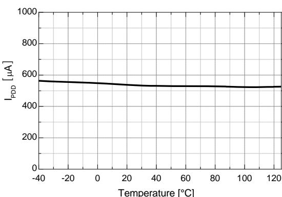
Figure 14. Operating  $V_{DD}$  Supply Current vs. Temp.
