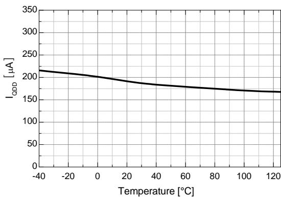
Figure 12. Quiescent  $V_{DD}$  Supply Current vs. Temp.
