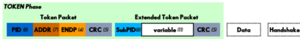
Figure 17 (above) : Extended Token Transaction
