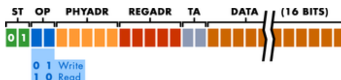
Figure 27 : Basic MDIO Frame Format
