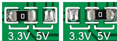
Button R click has a PWR SEL jumper [zero ohm resistor] that lets you switch between 3.3V and 5V power supplies.
