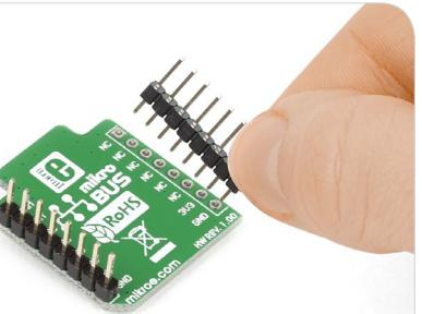
Turn the board upside down so that the bottom side is facing you upwards. Place shorter pins of the header into the appropriate soldering pads.
