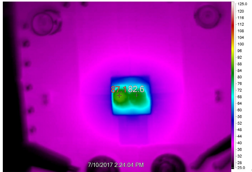
Figure 11. Thermal at V_{IN} = 12V , V_{OUT0} = 1.0V , I_{OUT0} = 25A , V_{OUT1} = 1.8V , I_{OUT1} = 25A , T_A = 25^{\circ}C , 200LFM Airflow
