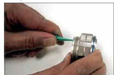
Plastic tool with contact in proper position.
