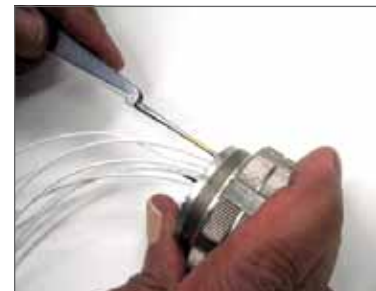
Removal of contacts with metal tool.
