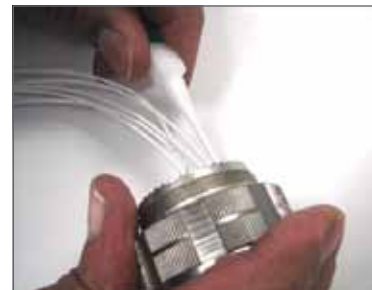
Use white end of plastic tool for removal of contacts.
