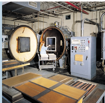
Heat-treating, critical to imparting the specific mechanical qualities to the spring materials, is computer-controlled. All heat treated batches are also quality tested for hardness and specifications.
