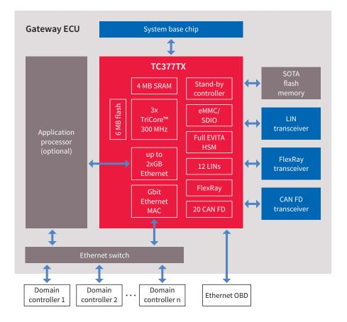
In gateway applications, AURIX<sup>™</sup> TC3xx microcontrollers support the latest communications interfaces and feature a Gigabit Ethernet interface, up to 12 ISO 11898-1-compliant CAN FD channels and up to 24 LIN channels. An additional eMMC interface for external flash interfacing enables local data storage, supporting software-over-the-air update concepts.
