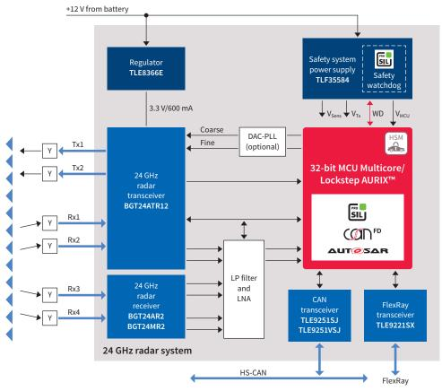
The new TriCore<sup>™</sup> AURIX<sup>™</sup> family will enhance classic safety features with dedicated features to meet the needs of 24 GHz radar systems. The combination of new features and increased SRAM, in conjunction with outstanding safety features, enables a high level of integration and reduction of complexity.
