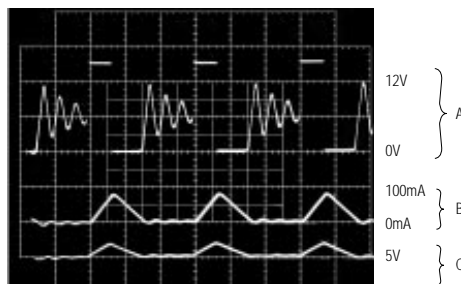
MAX758A SWITCHING WAVEFORMS DISCONTINUOUS CONDUCTION
