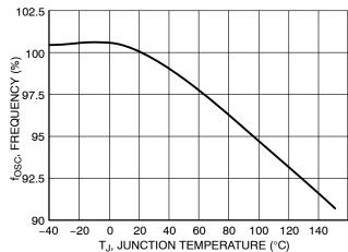
Figure 4. Oscillator Frequency Versus Junction Temperature
