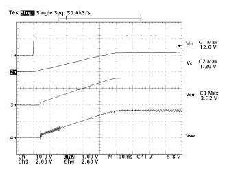
Figure 11. The Power Up Transition of NCV8843
