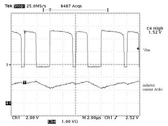
Figure 8. The Regulator in Current Limit
