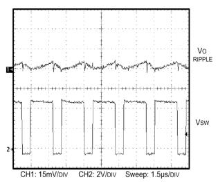
Figure 16. Output Voltage Ripple Using One 100 μF POSCAP Capacitor
