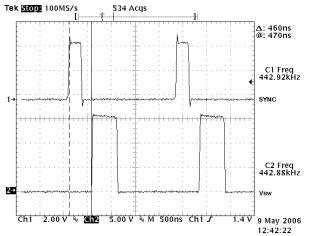
Figure 6. A NCV8843 Buck Regulator is Synchronized to an External 443 kHz Pulse Signal
