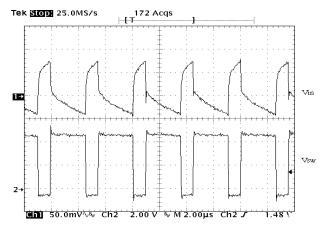
Figure 13. Input Voltage Ripple in a Buck Converter
