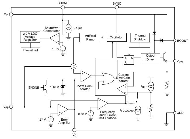
Figure 2. Block Diagram
