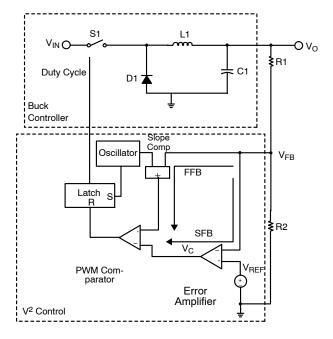
Figure 3. Buck Converter with V<sup>2</sup> Control.
