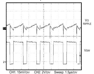
Figure 17. Output Voltage Ripple Using One 100  $\mu$ F OS–CON
