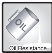
Oil Resistance (Insulation service life): twice or three times that of oil-resistant vinyl chloride
