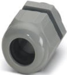
Cable gland, Cable gland material: Polyamide, External cable diameter 5 mm ... 10 mm, Shielding: No, Connecting thread: Pg11, Color: silver grey
