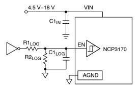
Figure 32. Logic Turn-on
