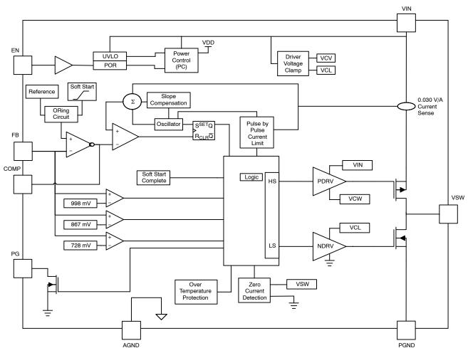
Figure 2. NCP3170 Block Diagram
