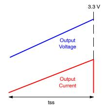
Figure 49. Resistive Load Current
