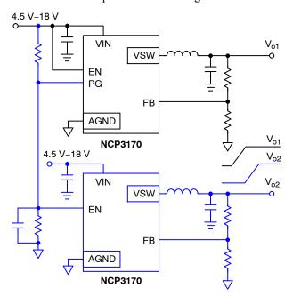
Figure 33. Enable Two Converter Power Sequencing
