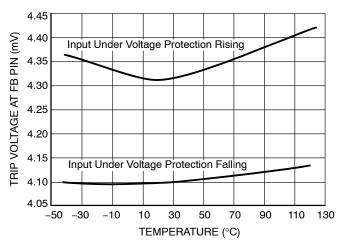
Figure 19. Input Under Voltage Protection vs. Temperature
