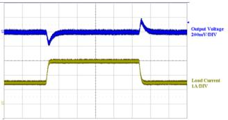
Figure 7. 50% to 100% Load Transient 100  $\mu s/\text{DIV}$
