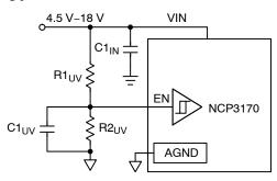
Figure 29. Input Under Voltage Lockout Enable
