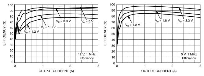
Figure 24. 12 V, 1 MHz Efficiency
