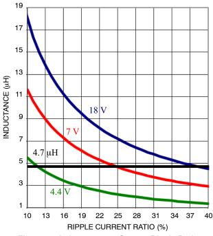
Figure 43. Inductance vs. Current Ripple Ratio
