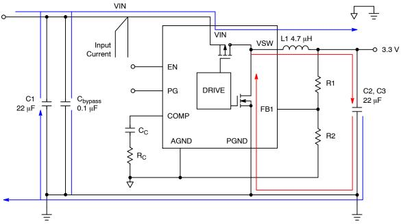
Figure 51. Buck Converter Current Paths
