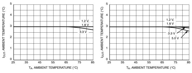
Figure 26. 1 MHz Derating Curves at 5 V Input
