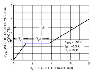
Figure 44. High Side MOSFET Total Charge
