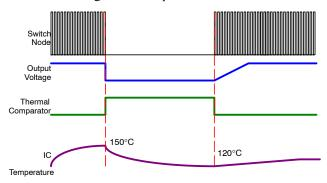
Figure 39. Over Temperature Shutdown
