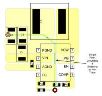
Figure 53. Recommend Thermal Layout
