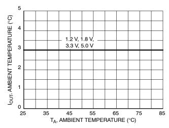
Figure 23. 500 kHz Derating Curves at 12 V
