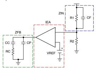
Figure 45. Pseudo Type III Transconductance Error Amplifier
