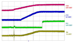
Figure 5. Start-Up into Full Load 1 ms/DIV
