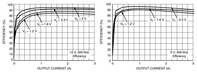
Figure 20. Efficiency (V<sub>IN</sub> = 12 V) vs. Load Current
