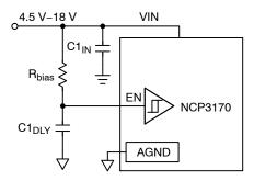
Figure 30. Delay Enable
