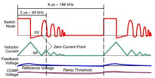
Figure 37. Light Load Operation
