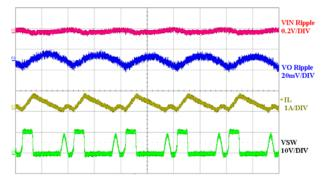
Figure 3. Light Load (DCM) Operation 1  $\mu s/DIV$
