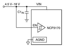
Figure 28. Input Voltage Enable
