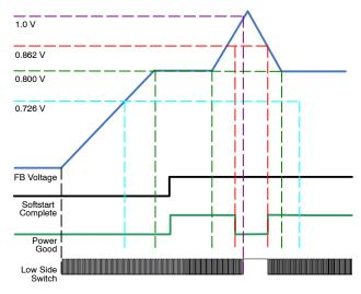
Figure 40. Over Voltage Low Side Switch Behavior
