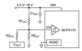
Figure 31. Added Hysteresis to the Enable UVLO
