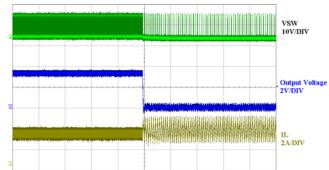
Figure 6. Short–Circuit Protection 200  $\mu s$  /DIV
