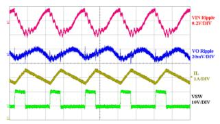
Figure 4. Full Load (CCM) Operation 1 μs/DIV
