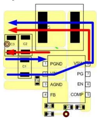
Figure 52. Recommended Signal Layout
