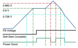
Figure 36. OOV and OUV Diagram
