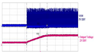
Figure 8. 3.3 V Turn on into 1 V Pre-Bias 1 ms /DIV
