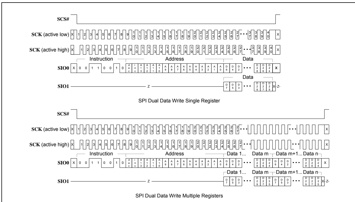
FIGURE 10-13: SPI DUAL DATA WRITE
