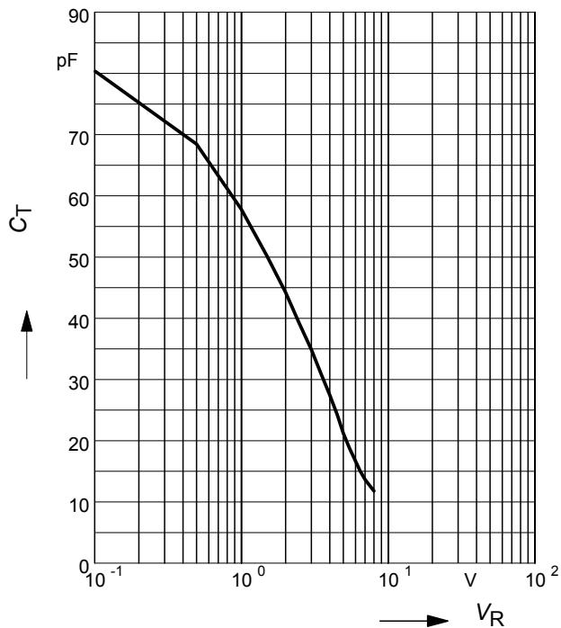
**Capacitance ratio  $C_{Tref}/C_T = f(V_R)$**
