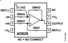
Figure 2. AD629 High Common-Mode Voltage Difference Amplifier
