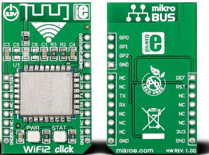
WiFi2 click™ is an affordable solution for adding WiFi functionality to your design. The board carries the **HLK-M30 WiFi module**, based on the universal serial interface network standard, with a built-in TCP/IP protocol stack. WiFi2 click™ is simple to use and is especially convenient for IoT applications. It communicates with the target board microcontroller through **mikroBUS™** UART (TX, RX) RST, and AN lines. It uses a 3.3V power supply.
