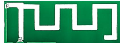
WiFi 2 click™ features a PCB trace antenna, designed for the 2400-2483.5 MHz frequency band.
