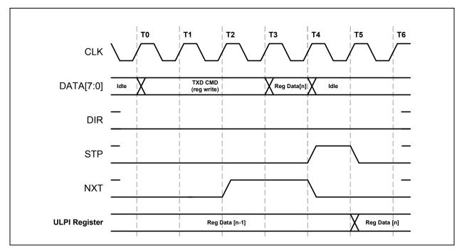
Figure 6.3 ULPI Register Write in Synchronous Mode
