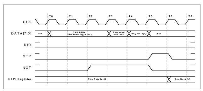
Figure 6.4 ULPI Extended Register Write in Synchronous Mode
