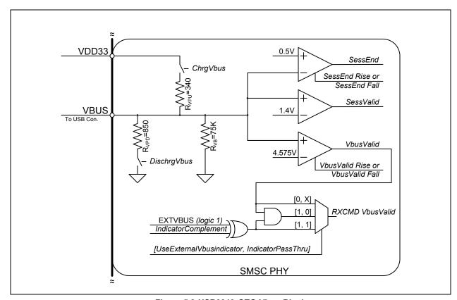
Figure 5.8 USB3319 OTG Vbus Block
