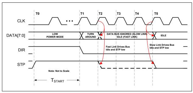
Figure 6.10 Exiting Low Power Mode
