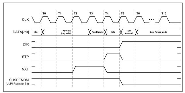
Figure 6.9 Entering Low Power Mode from Synchronous Mode
