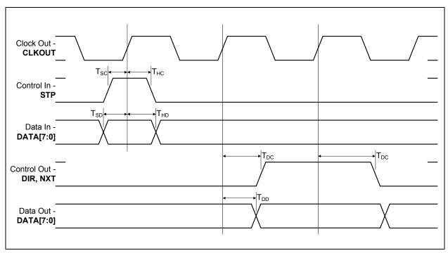
Figure 6.2 ULPI Single Data Rate Timing Diagram in Synchronous Mode
