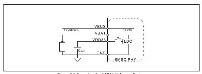
Figure 5.3 Powering the USB3319 from a Battery
