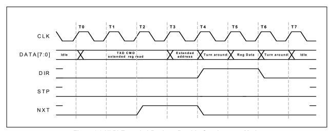
Figure 6.6 ULPI Extended Register Read in Synchronous Mode
