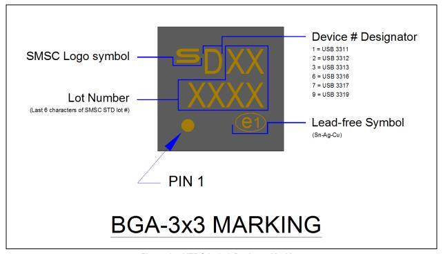
Figure 9.7 VFBGA, 3x3 Package Marking
