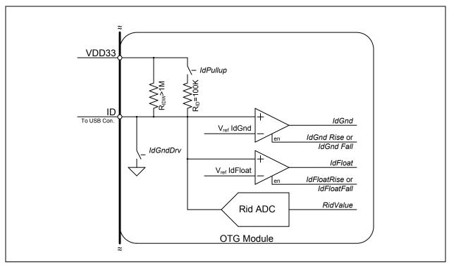
Figure 5.7 USB3319 ID Resistor Detection Circuitry
