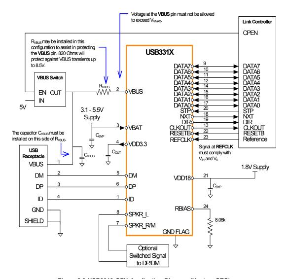
Figure 8.3 USB3319 QFN Application Diagram (Host or OTG)
