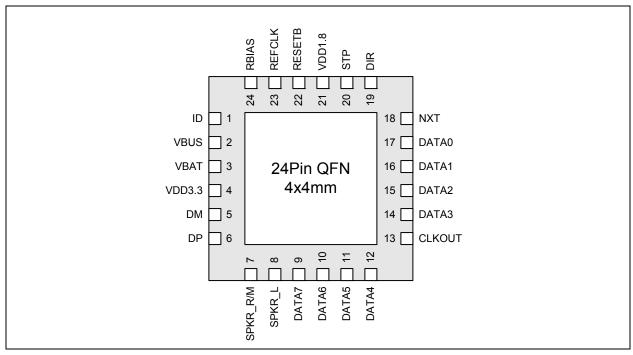
Figure 2.1 USB3319 QFN Pinout - Top View
