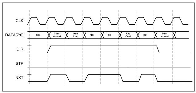
Figure 6.8 ULPI Receive in Synchronous Mode
