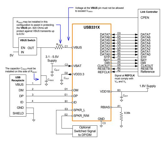
Figure 8.4 USB3319 BGA Application Diagram (Host or OTG)
