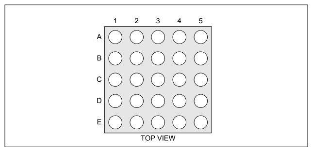
Figure 2.2 USB3319 VFBGA Pinout - Top View
