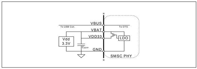
Figure 5.4 Powering the USB3319 from a 3.3V Supply
