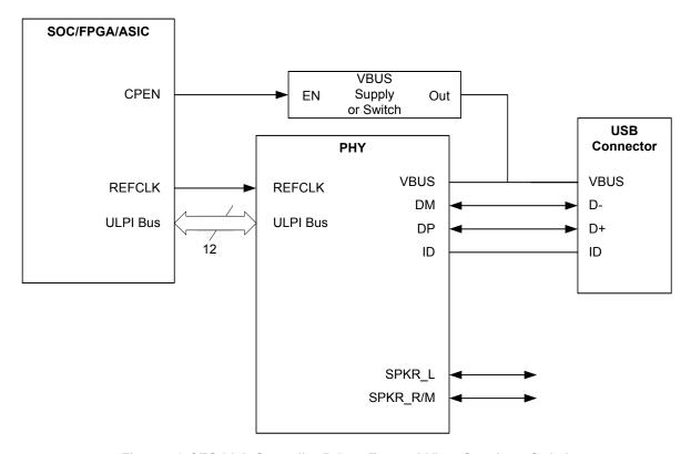
Figure 5.9 OTG Link Controller Drives External Vbus Supply or Switch
