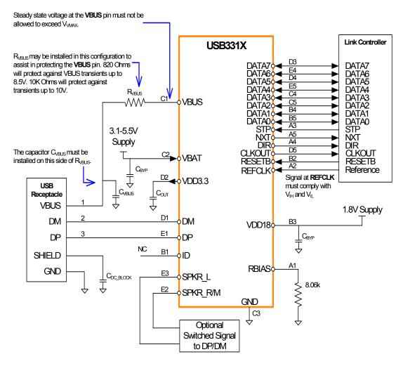
Figure 8.2 USB3319 BGA Application Diagram (Device)
