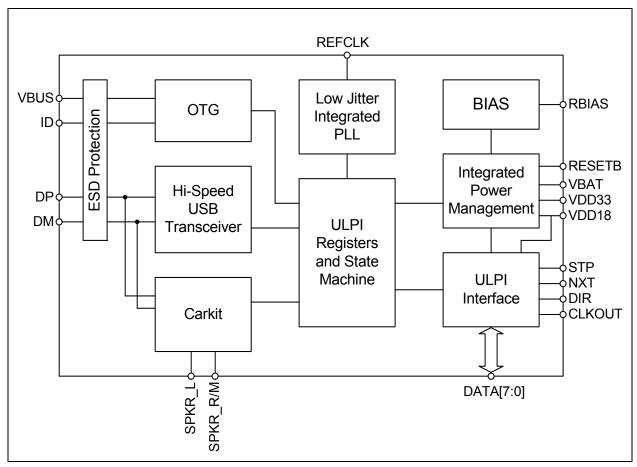
Figure 1.1 USB3319 Block Diagram
