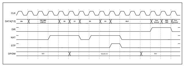
Figure 6.7 ULPI Transmit in Synchronous Mode
