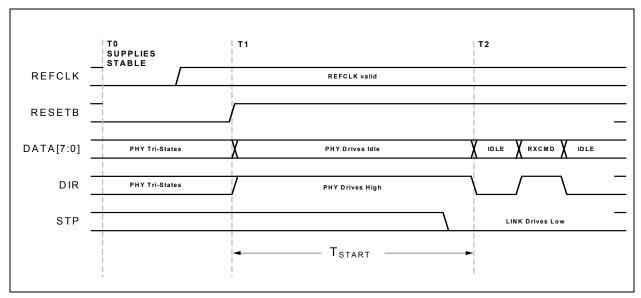
Figure 5.6 ULPI Start-up Timing
