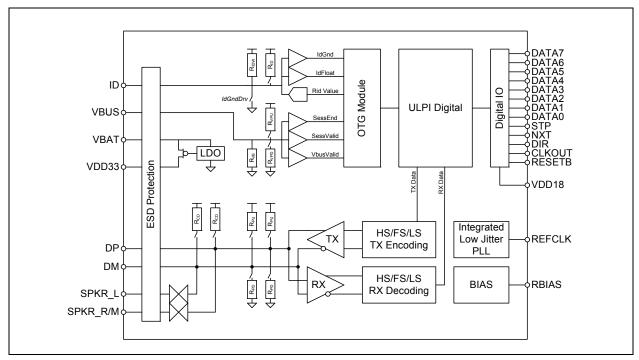
Figure 5.1 USB3319 System Diagram
