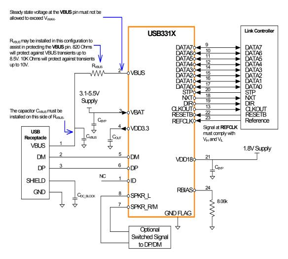
Figure 8.1 USB3319 QFN Application Diagram (Device)
