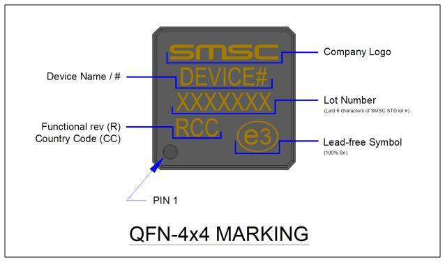
Figure 9.6 QFN, 4x4 Package Marking
