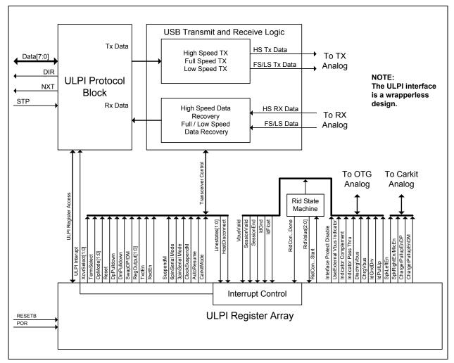
Figure 6.1 ULPI Digital Block Diagram
