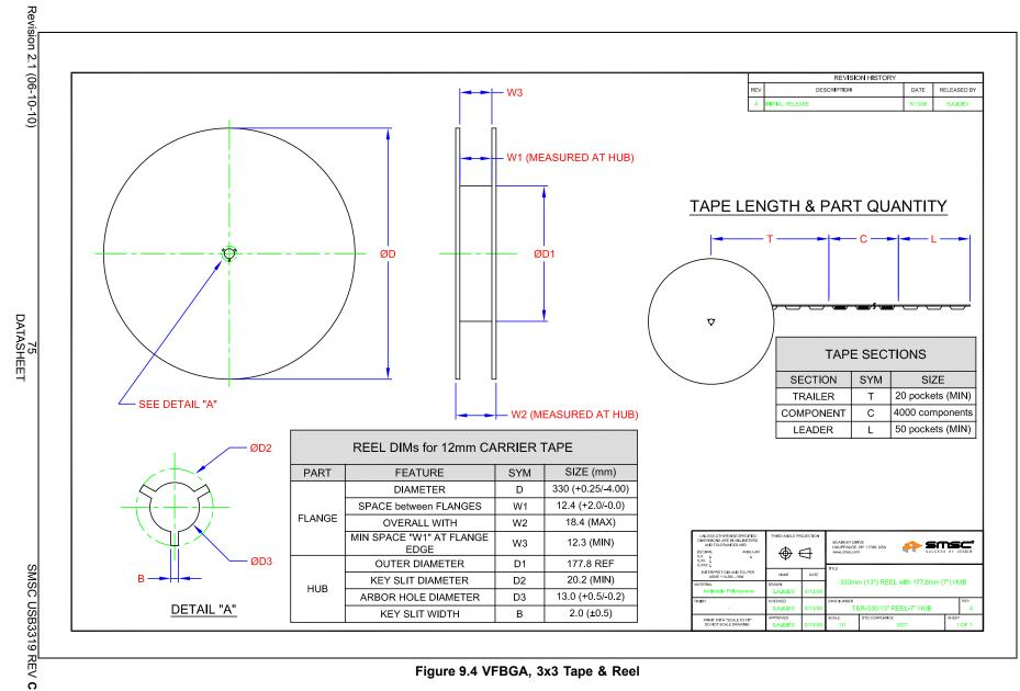
Figure 9.4 VFBGA, 3x3 Tape & Reel
