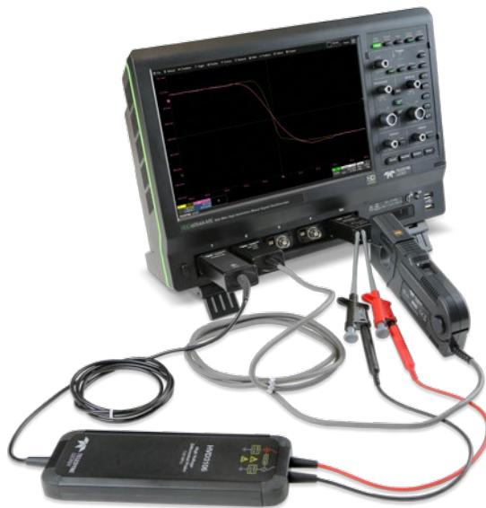
*CP150 150A current probe and HVD3106 high voltage differential probe connected to an HDO6104A-MS 12-bit resolution high definition oscilloscope. The DCS025 is connected to the EXT input (to conserve analog channels) and the deskew amount is adjusted for one of the probes in the channel dialog menu. In this case, a vertical Zoom of the current signal is used for deskewing.*
