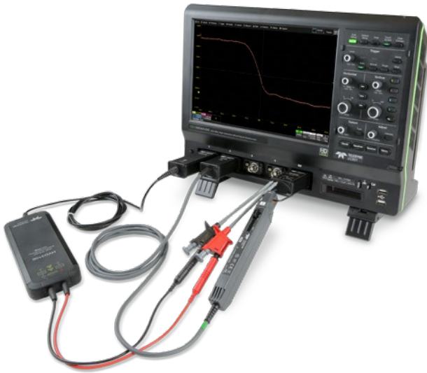
CP030 30A current probe and HVD3106 high voltage differential probe connected to an HDO6104A-MS 12-bit resolution high definition oscilloscope. The DCS025 is connected to the EXT input (to conserve analog channels) and the deskew amount is adjusted for one of the probes in the channel dialog menu.
