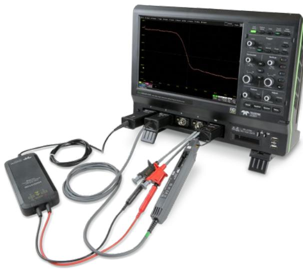
*CP030 30A current probe and HVD3106 high voltage differential probe connected to an HDO6104A-MS 12-bit resolution high definition oscilloscope. The DCS025 is connected to the EXT input (to conserve analog channels) and the deskew amount is adjusted for one of the probes in the channel dialog menu.*
