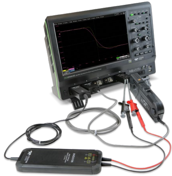
CP150 150A current probe and HVD3106 high voltage differential probe connected to an HDO6104A-MS 12-bit resolution high definition oscilloscope. The DCS025 is connected to the EXT input (to conserve analog channels) and the deskew amount is adjusted for one of the probes in the channel dialog menu. In this case, a vertical Zoom of the current signal is used for deskewing.
