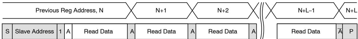
Figure 42. Sequential READ, Start from Current Location
