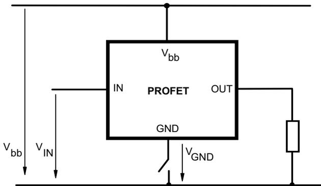
**V<sub>bb</sub> disconnect with charged inductive load**
