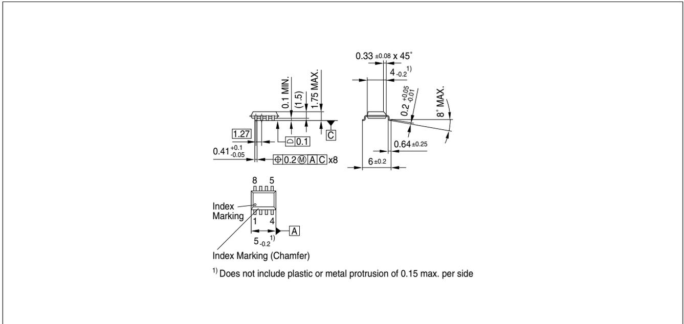
**Figure 1** PG-DSO-8-24 (Plastic Dual Small Outline Package) (RoHS-compliant)
