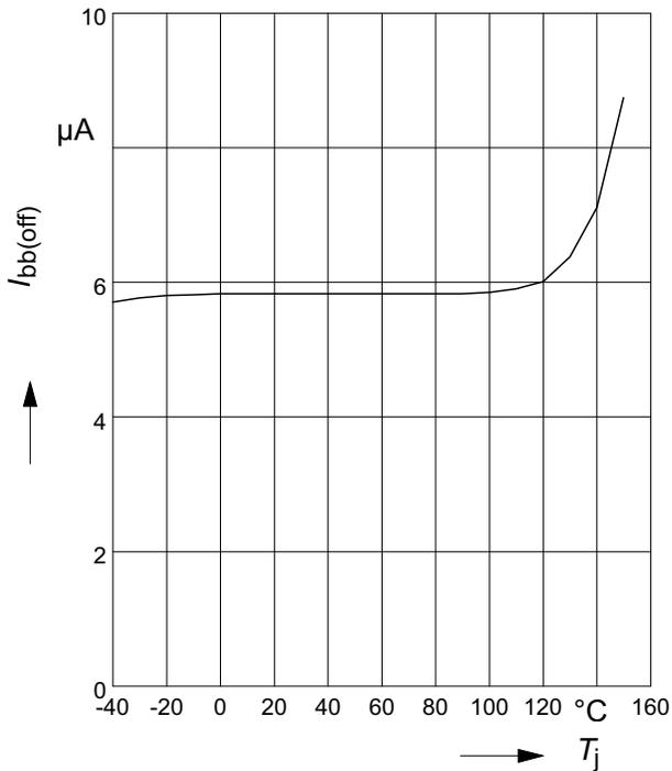
**Typ. leakage current**
