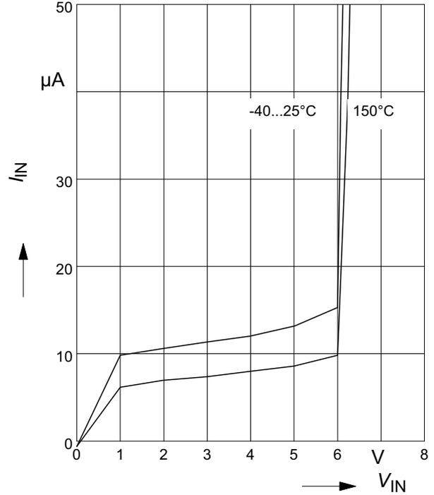
**Typ. input threshold voltage**
