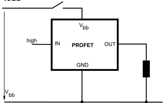
**GND disconnect with GND pull up**
