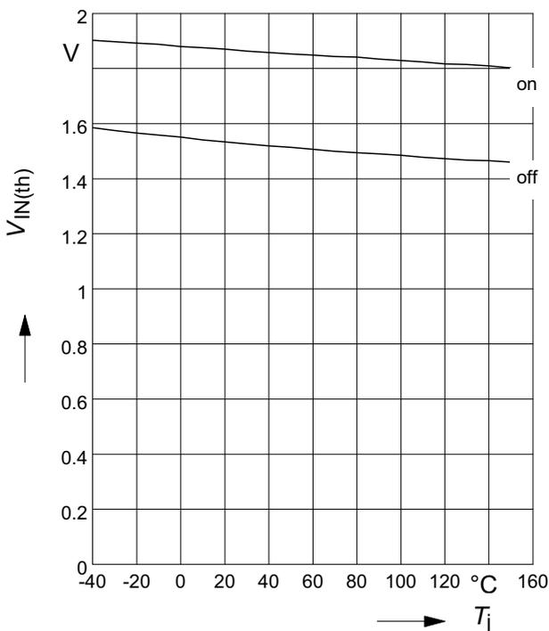
**Typ. input threshold voltage**
