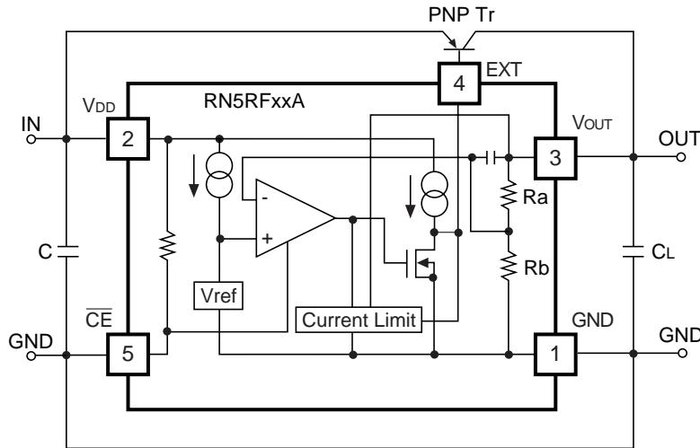
In these ICs, Output Voltage  $V_{OUT}$  is detected by feed-back resistors,  $R_A$  and  $R_B$  and the detected output voltage is compared with a reference voltage by the error amplifier so that the base current of an external PNP Transistor can be adjusted and the output voltage  $V_{OUT}$  is able to be regulated.
