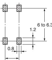
\* The external dimensions are different from those of the standard SOP 4-pin, but the mounting pad dimensions are the same.
