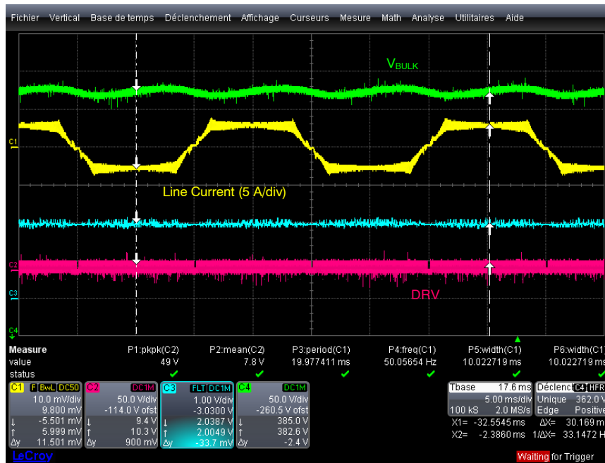
Figure 14. Over-Current Situation (85 V, 0.5 A Load Current)
