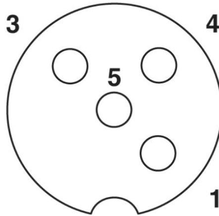
Pin assignment socket M 12, 3-pos. + PE
