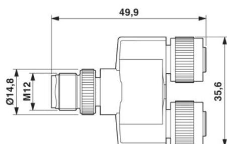
Connector M12 x 1, Y distributor, inner gauge of 21 mm
