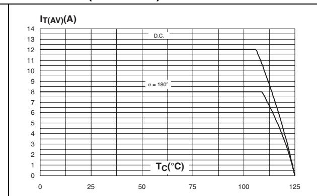
**Figure 3. Average and D.C. on-state current versus case temperature (TO-220FPAB)**
