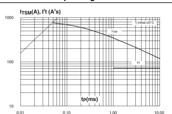
**Figure 9. On-state characteristics
