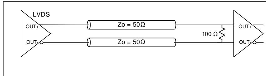
Figure 13. LVDS single DC termination at the load
