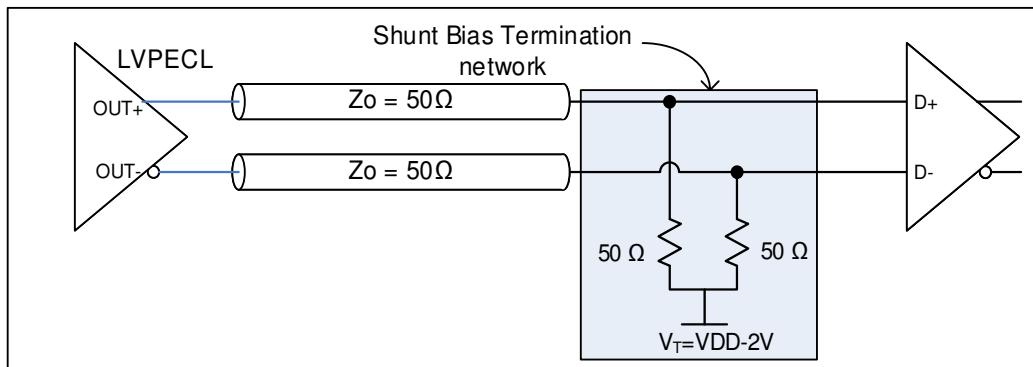
Figure 12. LVPECL with DC-coupled parallel shunt load termination
