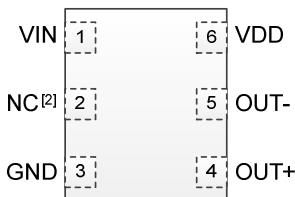
**Figure 2. Pin Assignments**
