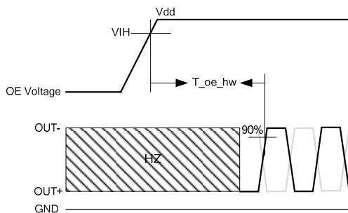
**Figure 7. Hardware OE Enable Timing**
