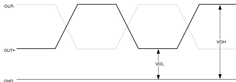
Figure 3. LVPECL/HCSL Voltage Levels per Differential Pin (OUT+/OUT-)
