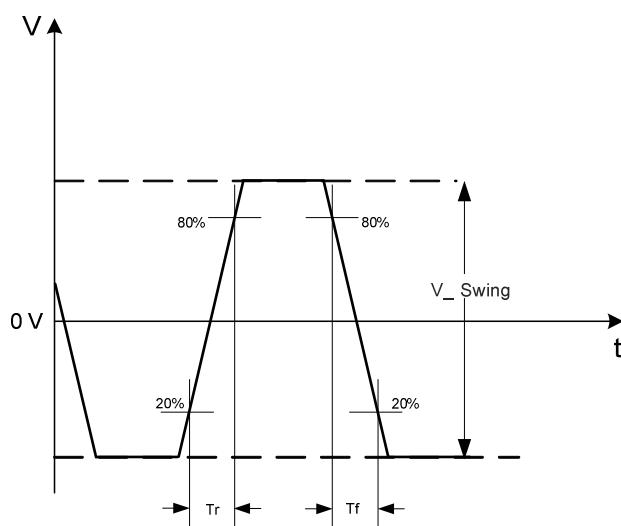
Figure 4. LVPECL/HCSL Voltage Levels across Differential Pair
