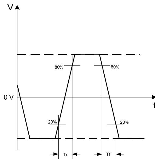
**Figure 6. LVDS Differential Waveform**
