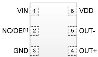
**Figure 1. Pin Assignments**
