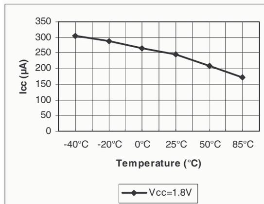
Figure 6. Icc vs. temp. Isink=2mA
