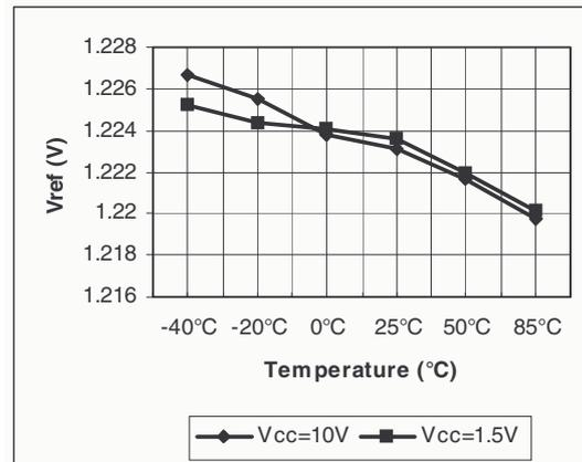
Figure 4. dVref/dVcc vs. temp. Isink=2mA
