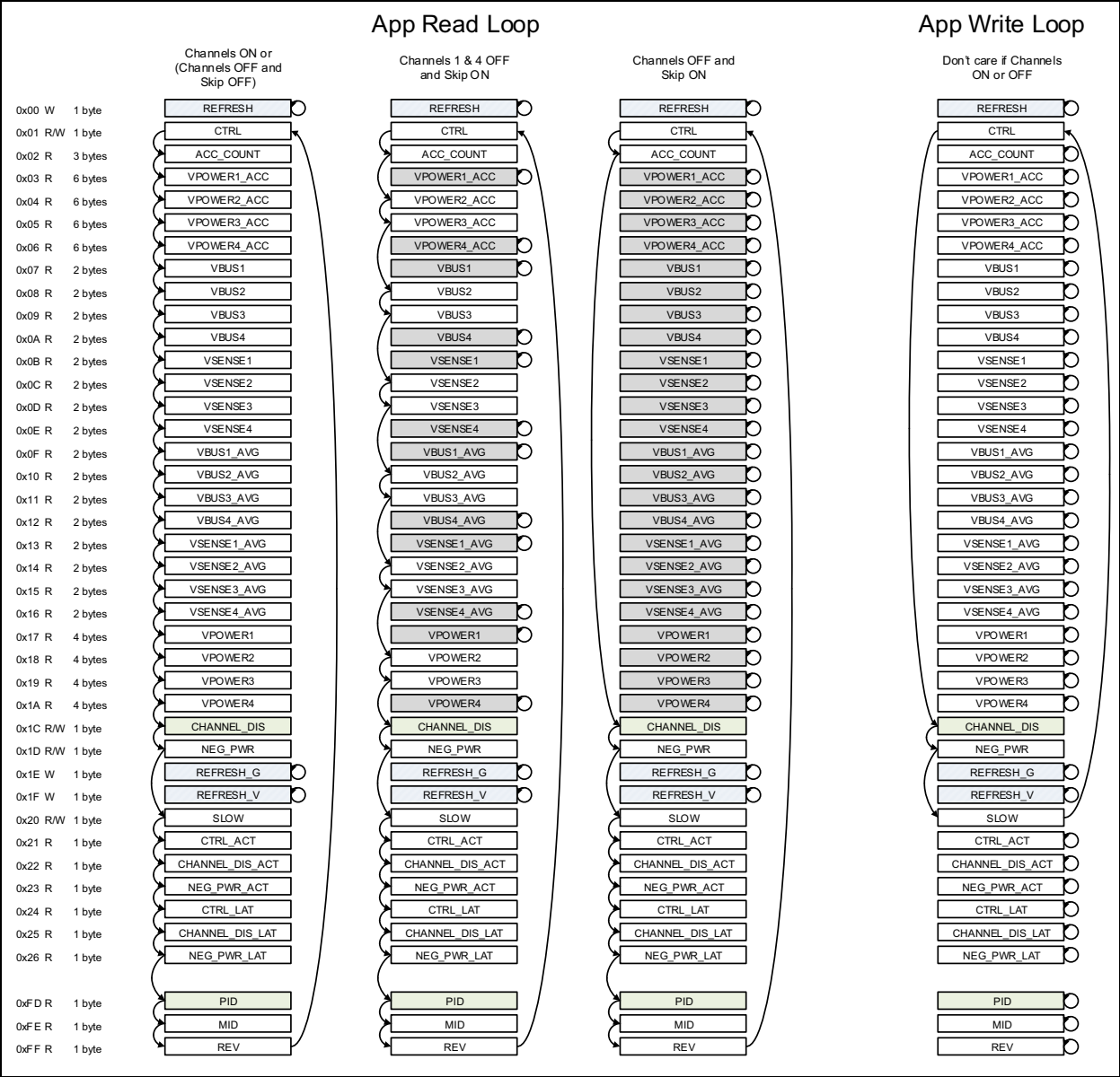
FIGURE 5-1: READ and WRITE Auto Incrementing Loops.
