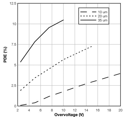
**Figure 3. PDE vs. Overvoltage**
