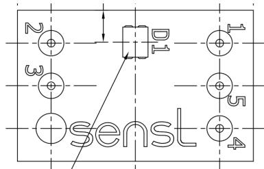
Figure 10. Top View of the SMTPA Board
