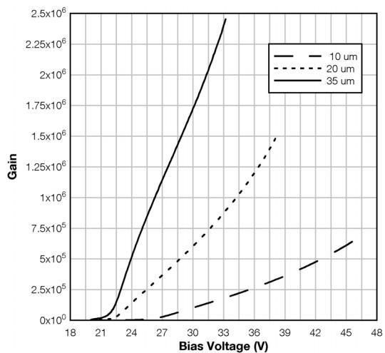
**Figure 4. Gain vs. Bias Voltage**
