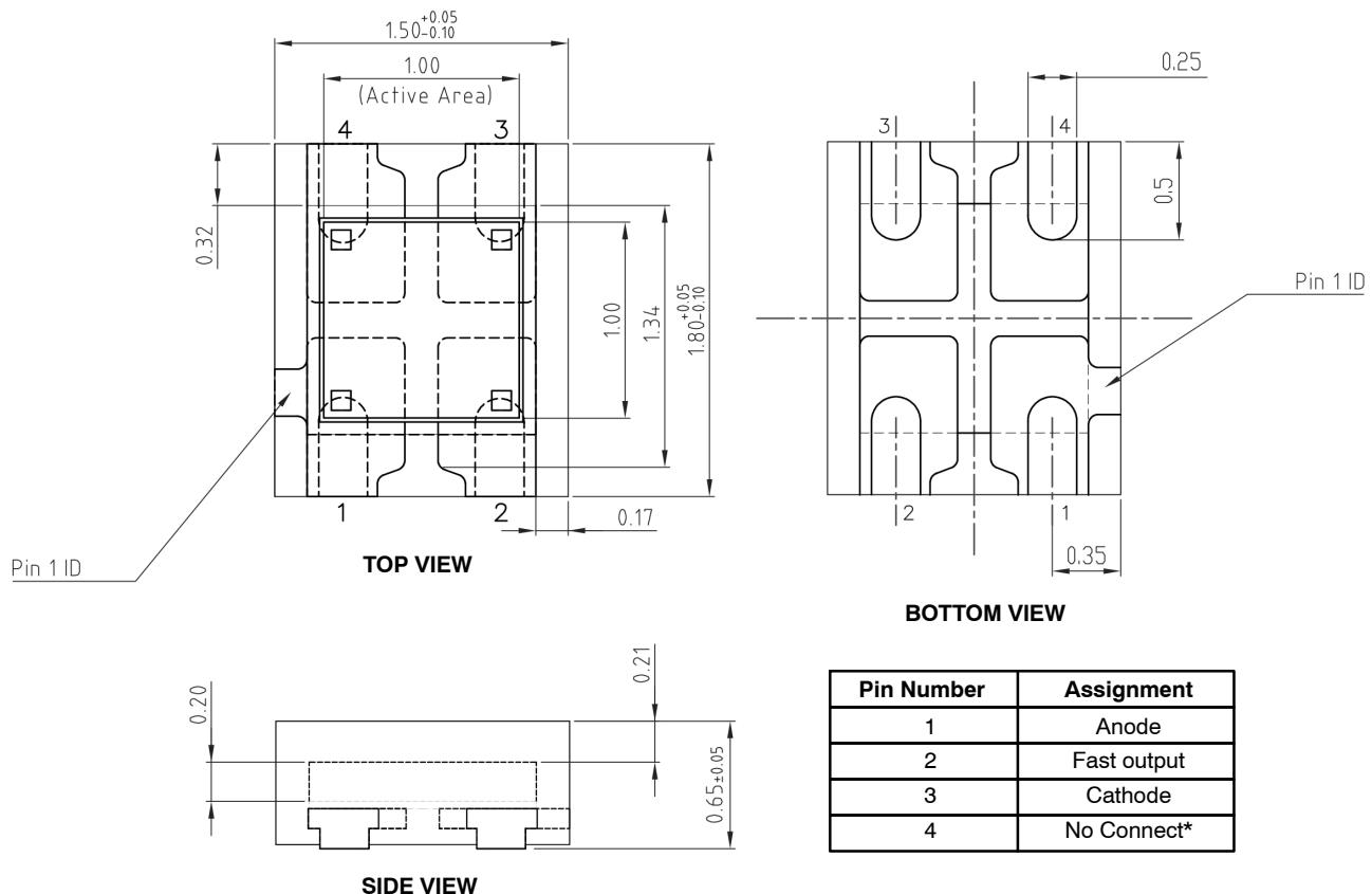
\*The 'No Connect' pins are electrically isolated and should be soldered to a ground (or bias) plane to help with heat dissipation.
