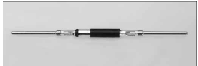
Close-up View of Diode Contact
