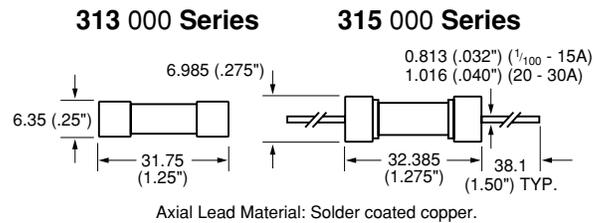
Axial Lead Material: Solder coated copper.
