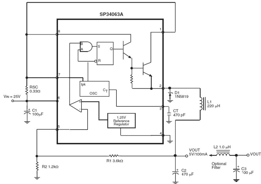
This is a typical buck converter configuration. The working process in the steady state is similar to a boost converter,  $V_{PIN5} = V_{OUT} \cdot R_2 / (R_1 + R_2) = 1.25(V)$ . The output voltage can be decided by  $V_{OUT} = 1.25V \cdot (R_1 + R_2) / R_2(V)$ .
