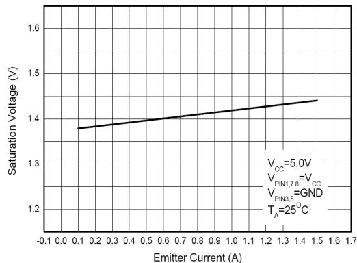
Fig. 8: Emitter Follower Configuration Output Switch
