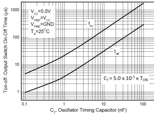
Fig. 4: Output Switch On-Off Time
