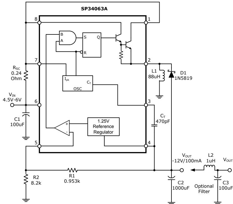
This is a typical boost converter configuration. The working process in the steady state is similar to a boost converter, the difference in this situation is that the voltage at the non-inverting pin of the comparator is equal to  $1.25V + V_{OUT}$ , then  $V_{PIN5} = V_{OUT} \cdot R_2 / (R_1 + R_2) = 1.25V, + V_{OUT}$ . The output voltage can be decided by  $V_{OUT} = -1.25V \cdot (R_1 + R_2) / R_1 (V)$ .
