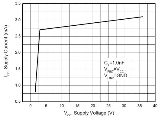
Fig. 7: Standard Supply Current vs. Supply Voltage
