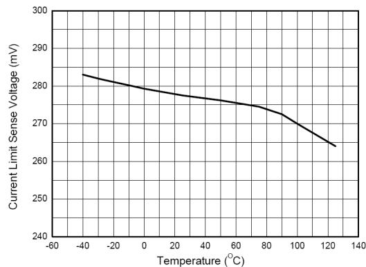
Fig. 10: Current Limit Sense Voltage vs. Temperature
