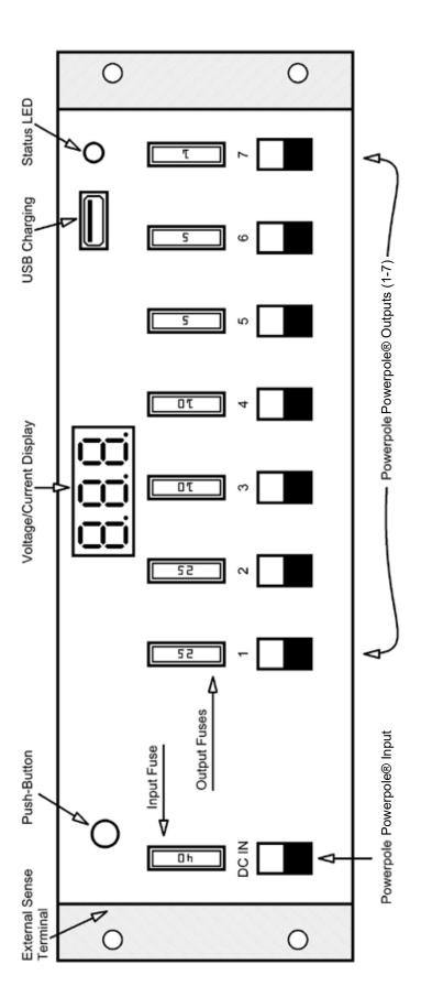
how many radios may be used to transmit at one time, consult the radio manual for power consumption specifications. In the event that the total current goes over the 40 amp maximum, a fuse will blow or make an undersized power supply unhappy. The RIGrunner and any equipment plugged into the RIGrunner should go unharmed.
