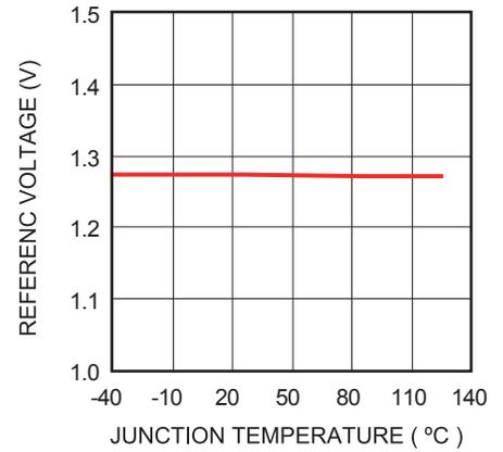
Enable ON/OFF Voltage vs.  $T_J$
