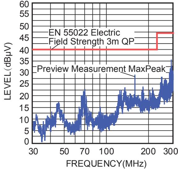
**Figure 5—EMI result,  $V_{in}=12VAC$ ,  $I_{out}=0.24A$ , 3LEDs, OATS**
