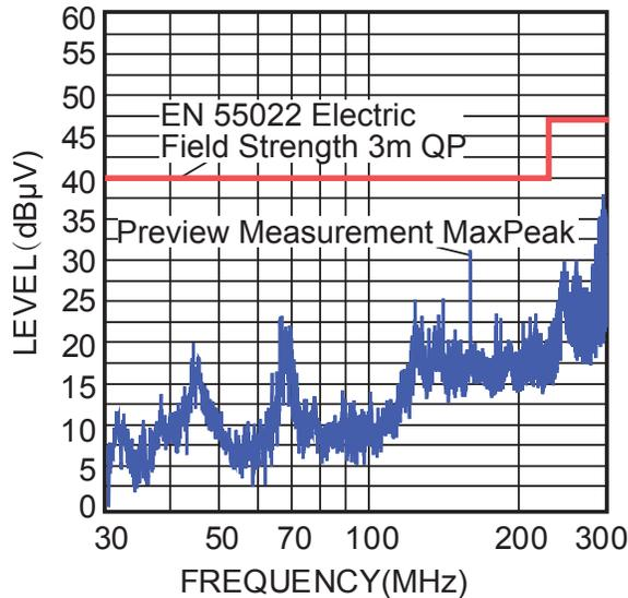
**Figure 6—EMI result,  $V_{in}=36VAC$ ,  $I_{out}=0.35A$ , 3LEDs, OATS**
