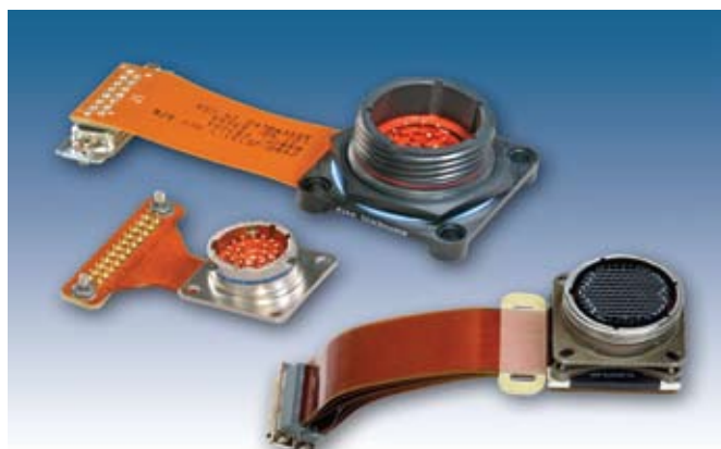
Flex Termination for Attachment to PC Boards
