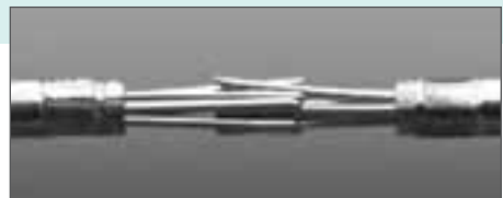
Bristle Brush Contacts - Multiple Stands of Wire are Bundled together to form a "Brush-like" Contact
