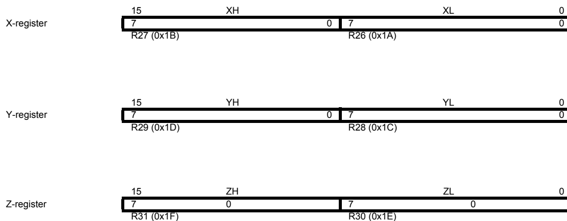
Figure 4-3. The X-, Y-, and Z-registers
